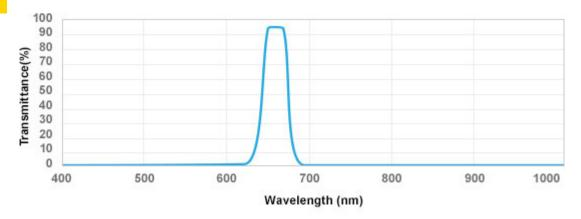
Function: Coated filter that transmits only specific wavelengths.
