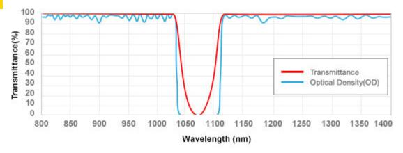
Function: It is a filter that attenuates light of a specific wavelength to a very low level and transmits light of other wavelengths.
