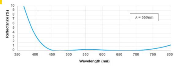
Function: Multilayer coating is used to limit the reflectance of a wide range as much as possible and increase the transmittance. It can also be used as surface protection.
