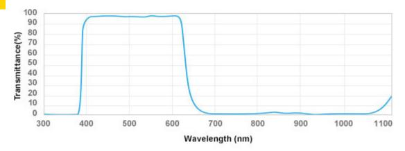
Function: It is a filter that transmits visible range and does not pass through ultraviolet range and near infrared range.
