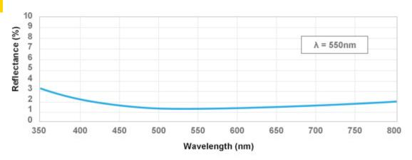
Function: Reduce the reflectance of a specific wavelength and increase the transmittance by using a single layer coating. It can also be used as surface protection.
