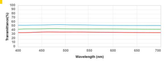
Function: It is a neutral density filter with a flat transmittance against wavelength.
